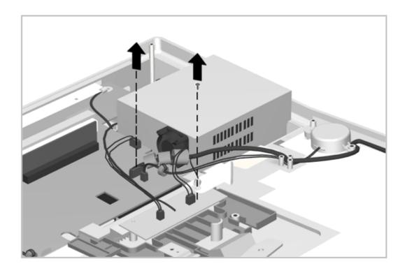
Figure 6-26. Disconnecting the IrDA Board
